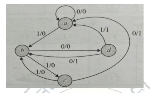
86. Design the sequence detector for the given state diagram using T flip flops.
