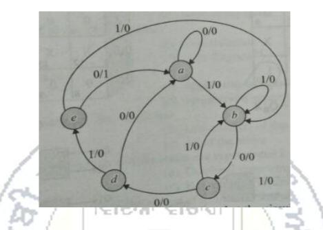
81. Design with D flip flop and JK flip flop the clocked sequential circuit whose state diagram
